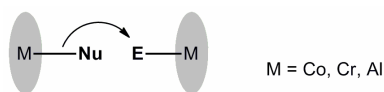
Figure 9. Schematic representation of cooperative activation of both nucleophile (Nu) and electrophile (E) by metallocalen catalysts.
