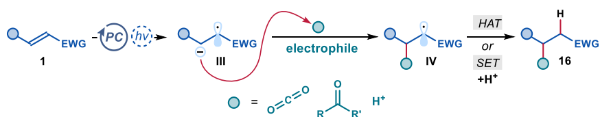
Figure 3.9. Photocatalytic generation of radical anion III via SET reduction of electron-poor olefins
