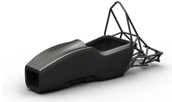
Figura 1.4. Xassís monocasc d'un vehicle de la Formula SAE. [ https://www.semanticscholar.org/paper/Analysis-of-Composite-Chassis-Eurenius-Danielsson/14f9d8e99cb1012baacf9239c89d7f4804544bb9#extracted ].
