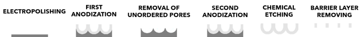
Figure 2. Effect on the aluminium at each step of the fabrication process. It starts with bare aluminium and continues with pore growth until it finally has open pores.
