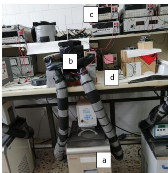
Figure 5. Assembly of the first anodization process: a) cooler, and b) PVC cell on top of the cooler and protected to maintain the temperature controlled by a thermometer, c) multimeter, and d) power source.
