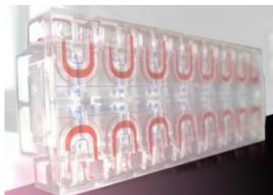
Figure 11. Patchliner chip (NPC-16). The external fluidic channel is indicated in red and the internal fluidic channel in blue [16].
