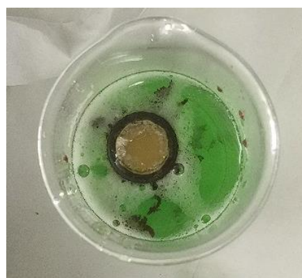
Figure 26: Alumina template being dissolved in HCl + \text{CuCl}_2 solution
