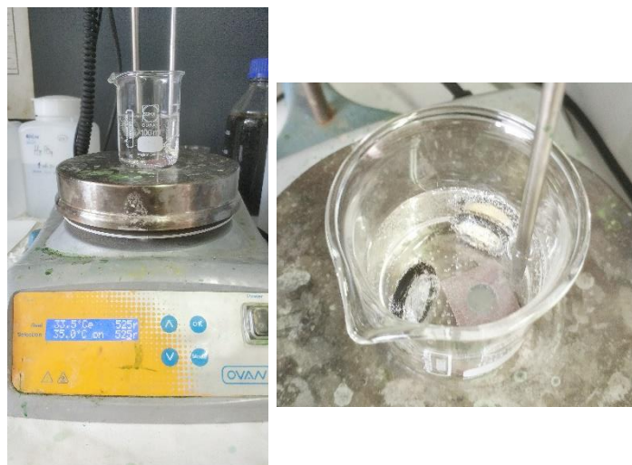
Figure 27: Polymeric replica immersed in phosphoric acid ( H_3PO_4 ) at 35 °C aprox.
