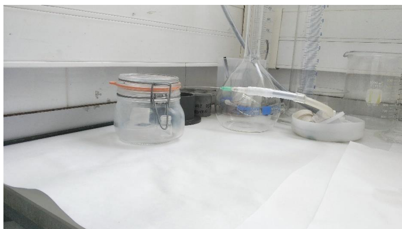
Figure 17: Coating of the macropSi surface with a layer of perfluorooctyltrichloro-silane
