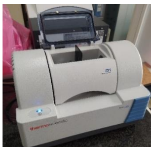
Figure 12. FT-IR Nicolet iS5 with transmittance accessory
