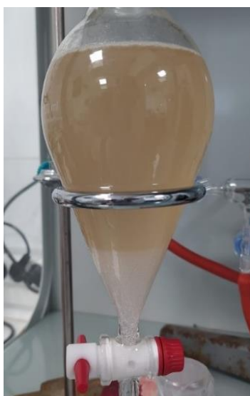
Figure 8. Wastewater sample extraction containing a high volume of emulsions.
