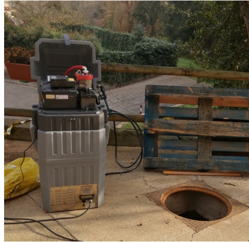
Figure 4 Automatic sampler equipment and deployment
