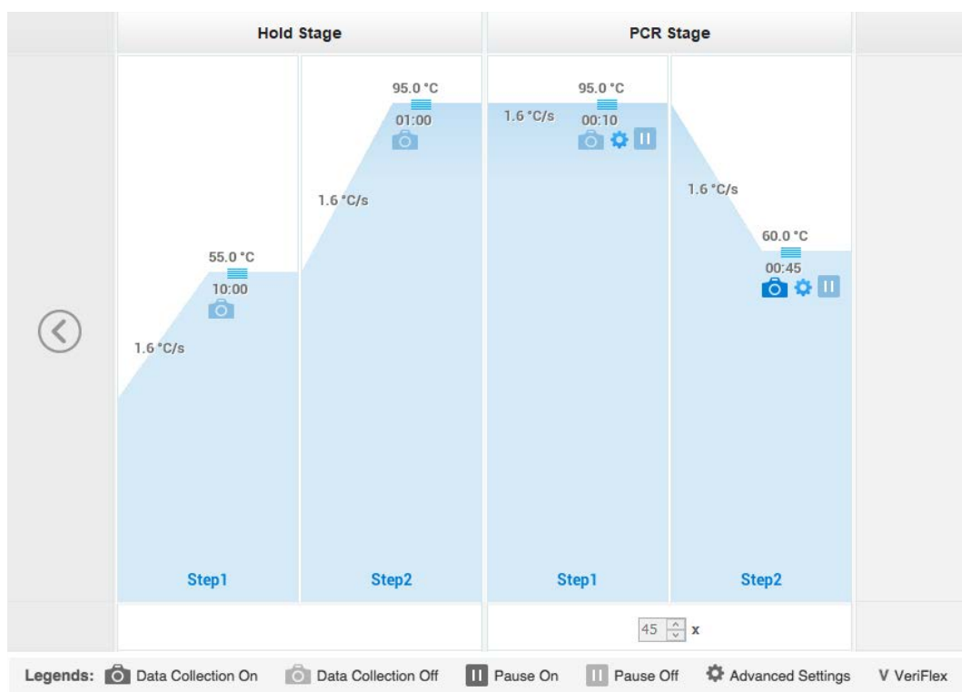
Figure 19. Schema of repeats, temperature and time conditions for each step of the RT-qPCR reaction. It is also illustrated when the instrument collects fluorescence information (final step).
