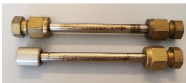
Figure 5. Two axial passive sampling tubes, the upper one with the two brass stoppers used to avoid contamination when not in use and the lower one with the diffusive cap on the corresponding end.
