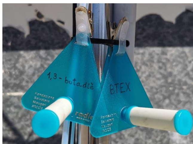
Figure 4. The two radial passive sampling tubes placed in their diffusive bodies and mounted on their support plates at the sampling point.
