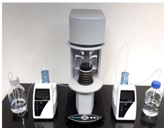
Figura 5.4 Force Tensiometer Sigma 700/701 . 24
