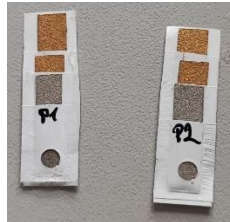
Figura 6 Primers sensors OECT de format totalment vertical
