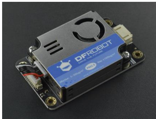
Figura 4.6. DFRobot Gravity: PM2.5 Air Quality Sensor. [41]
