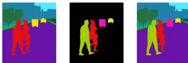
Figure 10. Types of segmentation, from left to right: semantic segmentation, instances segmentation and panoptic segmentation. [18]
