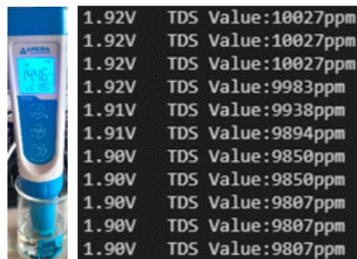
Figure 15. Conductivity measurement, and voltage and TDS measurements, respectively, in Ri-Lac solution
