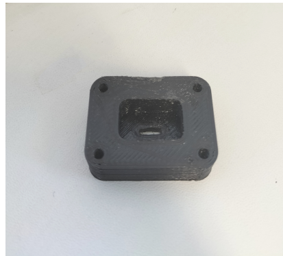
Figure 32. Cover manufactured with a 3D printer
