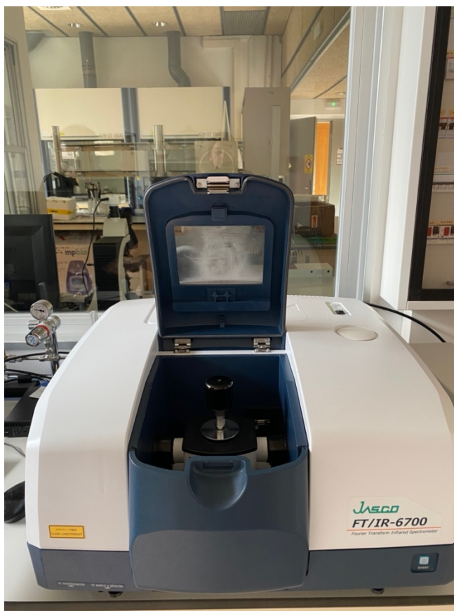
Figure 16. Jasco FT/IR-6700, used for recording IR spectra.
