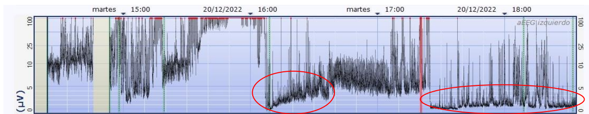
Figure 31: 2nd restriction, in which the aEEG presents narrow bands (red line). Rather than brain activity, this is attributed to a conductive bridge between the electrodes of the same hemisphere, obtaining the same input. (Case 1)
