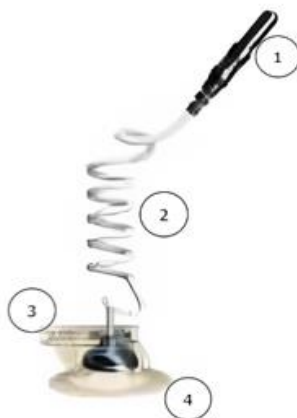
Figure 19: a-CUP electrode scheme. (1) Universal connector, able to connect to all EEG devices. (2) Coil of wire to facilitate movement without detachment. (3) Opening to introduce the gel, with its cover to avoid electroconductive gel spill. (4) Adhesive for delicate skins, long recordings, and good adherence.
