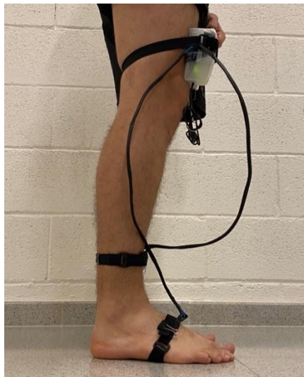
Figure 3. Ankle's set up with one MPU fixed on the toe and the other one on the leg. The microcontroller and the battery is on the distal anterolateral thigh.
