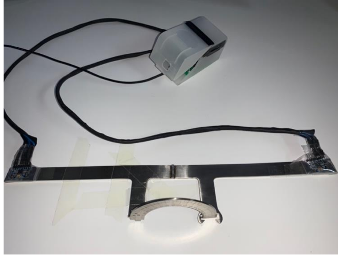
Figure 24. Stable position of the goniometer on the table with both sensors fixed with tape on it. The fix arm was also adhered on the table.
