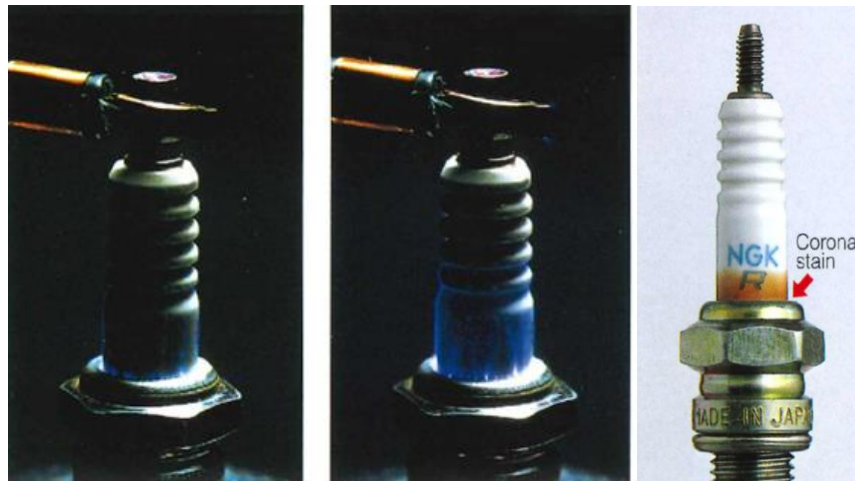
Figure 49 Corona discharge phenomenon and result [18]
