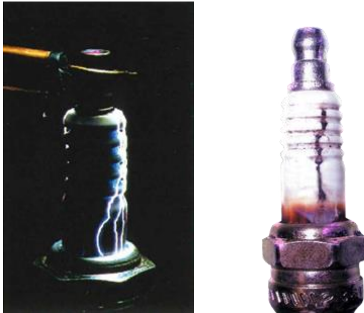
Figure 50 Flashover phenomenon and result (Left: [18], Right: [30])
