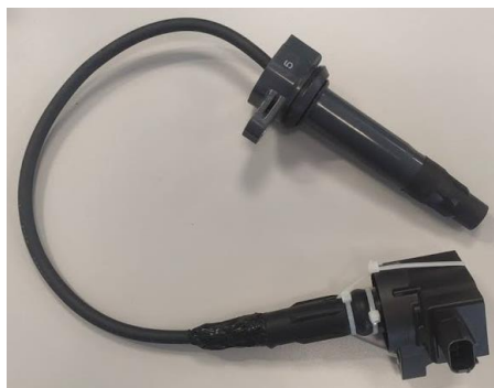
Figure 76 Adapter for high side output measurement
