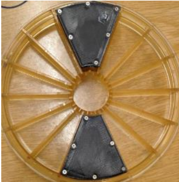
Figure 50 Endcap with two cut spokes and two Sensor Cover.
