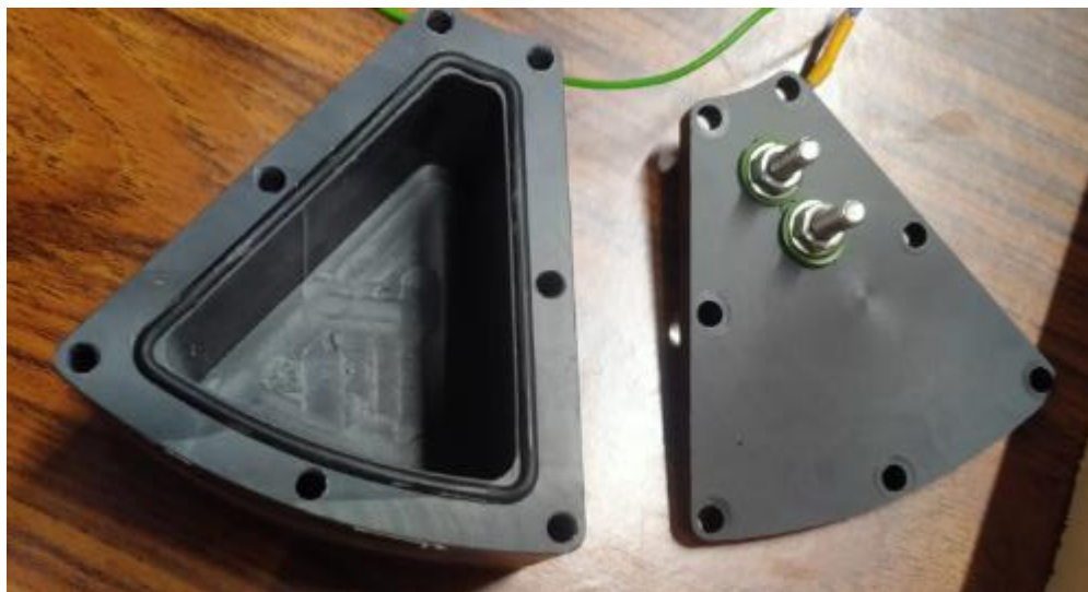
Figure 53 Final Sensor Cover with 2 electrodes.
