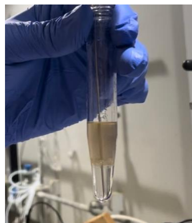
Fig. 7: Visualization of the two phases formed after water addition. Aqueous phase is in the upper part, while the organic phase is in the lower part.
