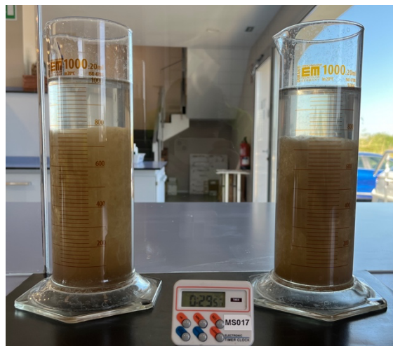
Figure 2. Column settling test.
