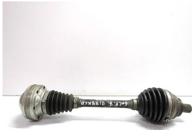
Figura 47 Palier de Volkswagen Golf 5p Sport R-Line 1.5 TSI EVO 110 kW (150 CV) DSG 7 vel. (2019-2020)[33]
