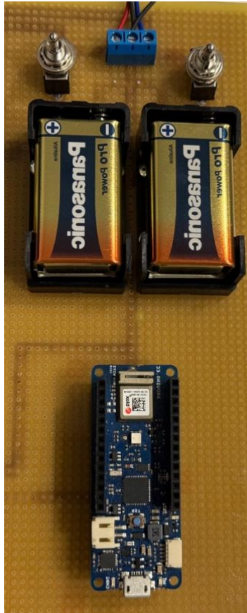
Figure 21. Power of the circuit, levers for the activation and the microcontroller, Arduino MKR1010.
