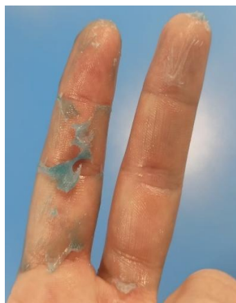
Figure 12. Comparison of sustained bending resistance between BPAG (left finger) and Reference 11 (right finger) applications.
