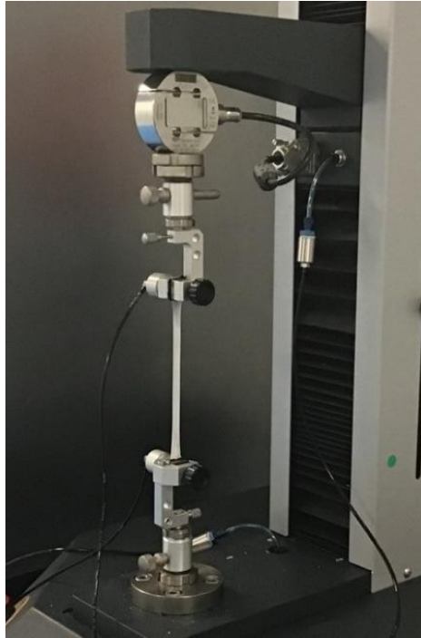
Figure 7. Tensile test of a film strip using the UTM.
