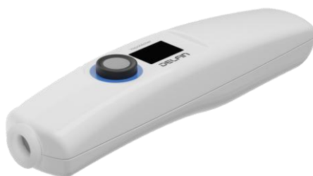
Figure 5. VapoMeter, a TEWL meter from Delfin Technologies.
