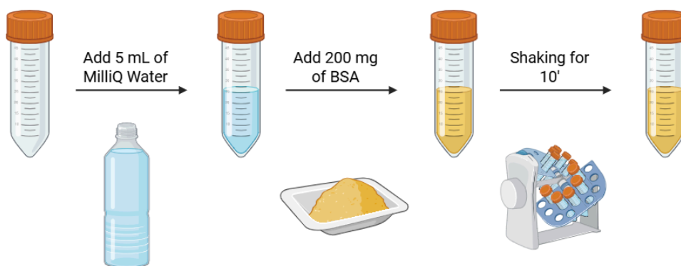
Figure 9. Methodology employed for the preparation of albumin 40 mg/mL. Generated by BioRender.
