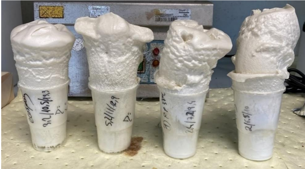
Figure 6. Example of free-rise spray foams
