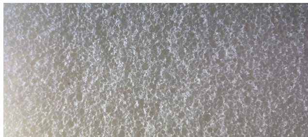
Figure 9. High open cell content on a flexible foam
