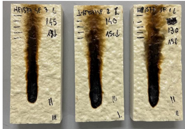
Figure 10. Example of three samples subjected to a flame behaviour test
