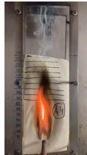
Figure 7. Small burner fire test
