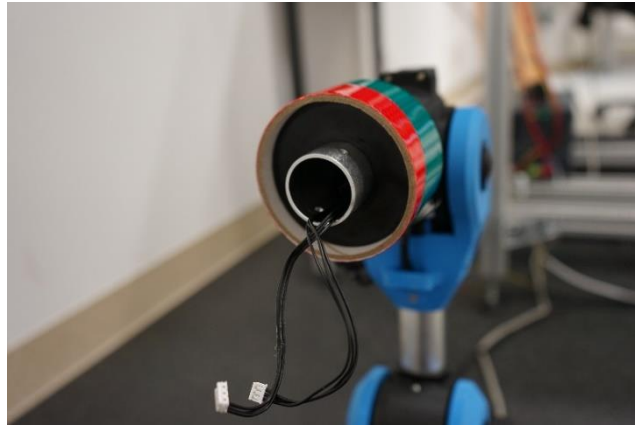
Figure 10 3D printed junction cylindrical piece.
