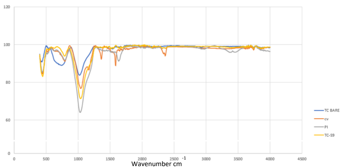
Figure S5: FTIR analysis of dye interactions and TCpSi. Legend: TC bare is bare TCpSi, and TC CV, TC PI and TC S9 are TCpSi stained with crystal violet, propidium iodide and SYTO 9, respectively.
