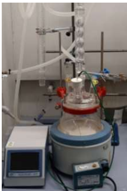
Figure 10: Scale-up set up for BMI.Cl and BISCAT.Cl synthesis
