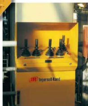
Hydraulic control console allowing the control of four hoist/trolley combinations
