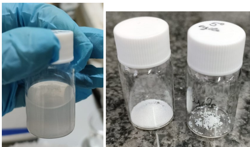
Fig. 34 Due to the enzyme leaching, there is the formation of turbidity in the reaction medium (a) and therefore reduction of the enzyme quantity (b)
