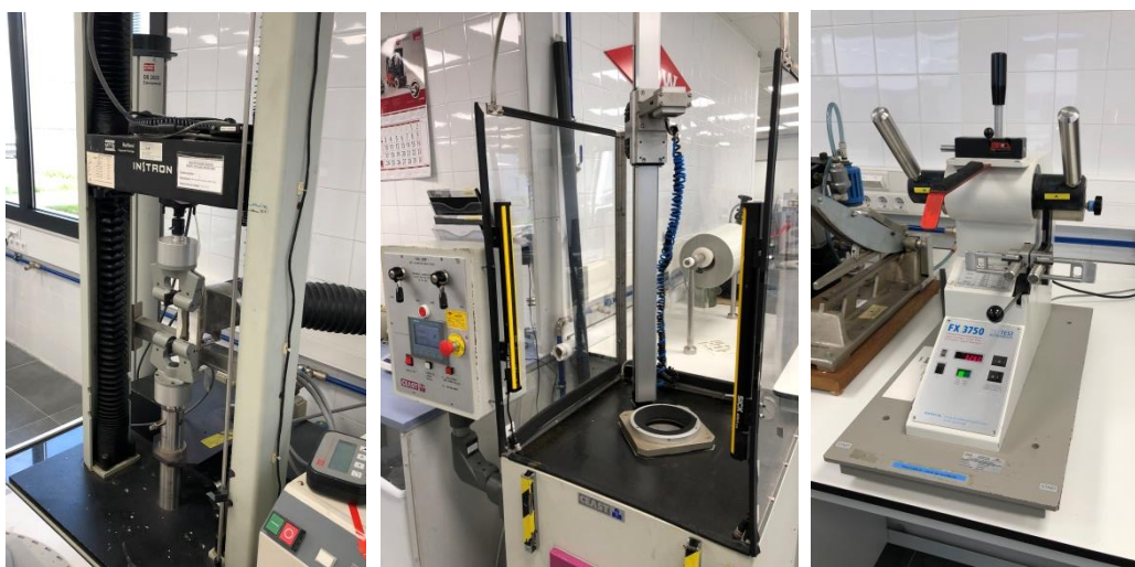
Figure AII.1. Tensile, Dart Drop Impact and Elmendorf tear machines. (Own source)
