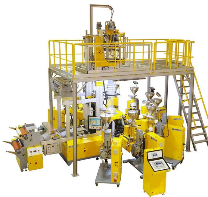
Figure 5.4. Coextrusion Blown – Collin 9L similar to the Tarragona Pack Studios one. (10)
