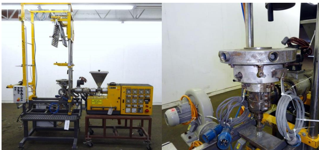
Figure 5.1. Extrusion Blown – Collin 30 mm similar to the Tarragona Pack Studios one. (9)
