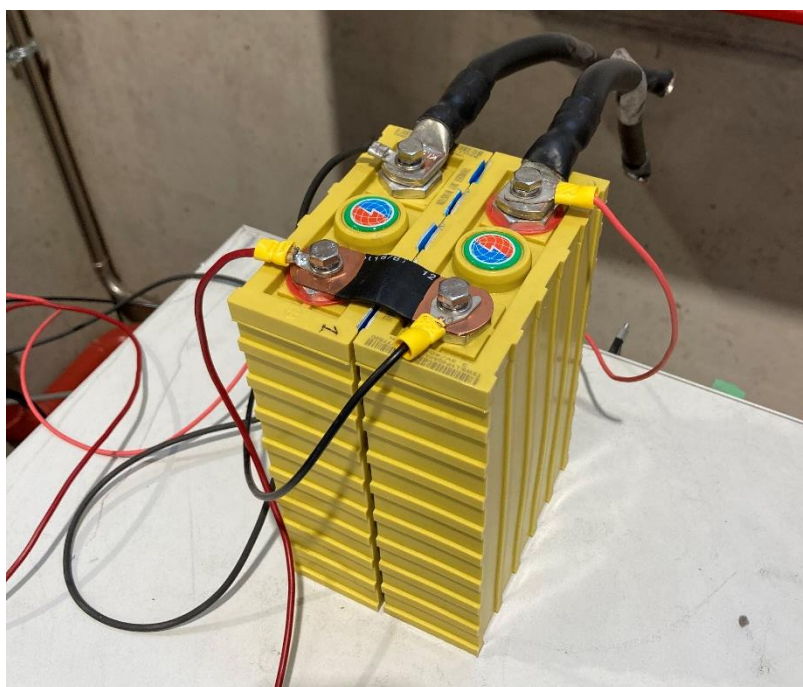
Figure 15: Two series-connected prismatic LFP cells
