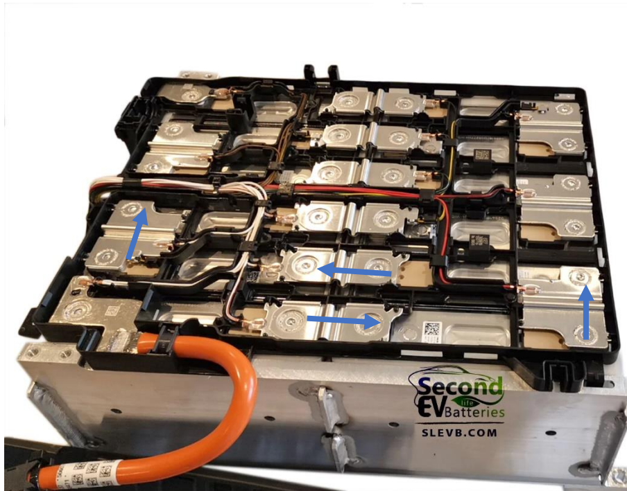
Figure 8. BMW I3 module, top plastic removed.
