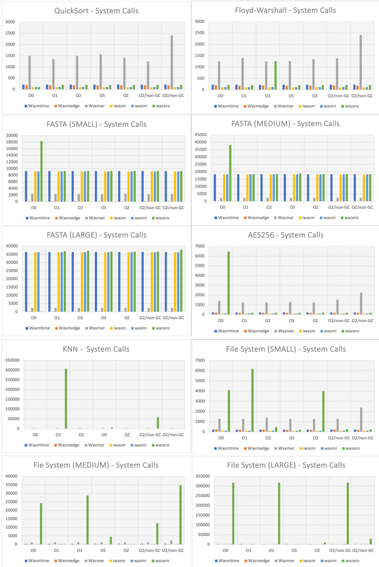
Figure 44. Number of System Calls for each benchmark and runtime. Generated by the author Safia Guellil.
