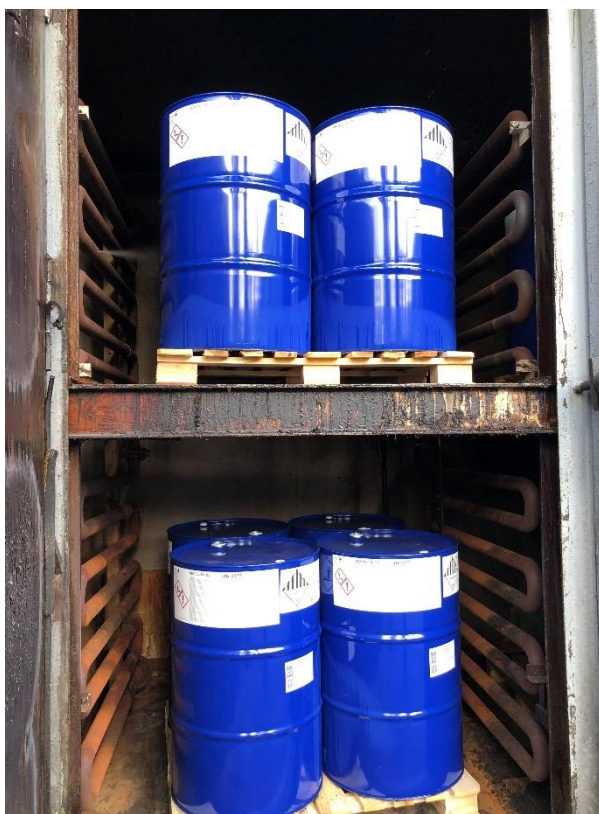
Figure 1. Picture of half of a fusion chamber in operation occupied by metal drums of product.
