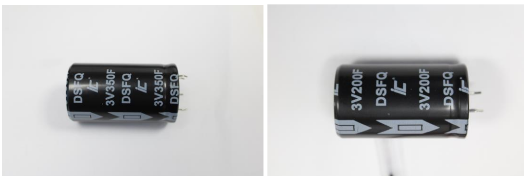
Figure 10. Cornell supercapacitors 3 V 350 F (left), 3 V 200 F (right)
