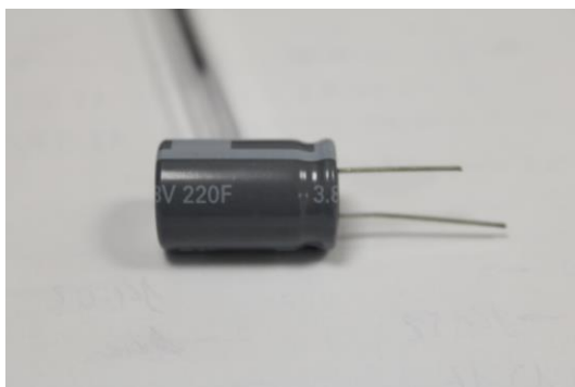
Figure 12. Eaton hybrid supercapacitor 3.8 V 220 F
