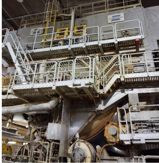
Figure 1.8. Yankee dryer and drying hood. Own work.
