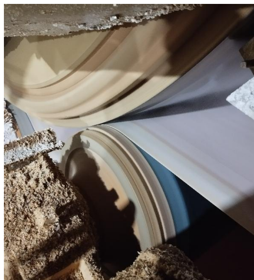
Figure 1.7. Dewatering produced due to Yankee dryer – blind press contact. Own work
