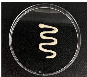
Figure 6 not-printable 2,5%TM stabilized HIPE.
