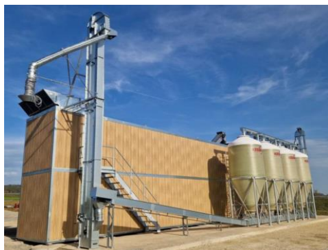
Figure 4.14 Natural Ventilation Dryer by Huber.
