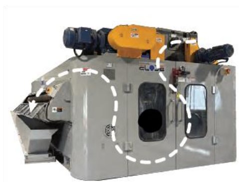
Figure 4.11 Electro-osmosis dryer by Bluewin.
