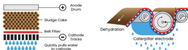
Figure 4.12 Operational principle of the electro-osmosis dryer. (Iwata et al., 2013)
