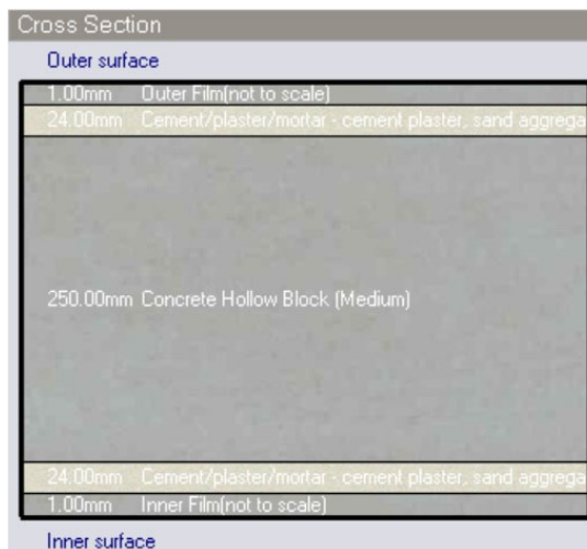
Figure 2-12(b): Baseline model, wall cross section
