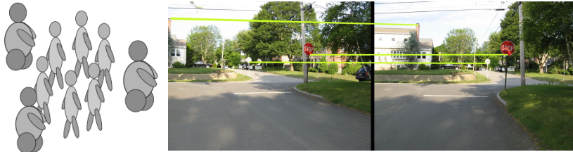
Figure 2. A representation of three robots performing guiding tasks and images taken from the cameras on the first two robots.
