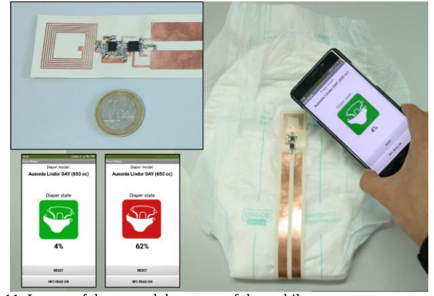
Fig.11. Layout of the tag and the screen of the mobile app.
