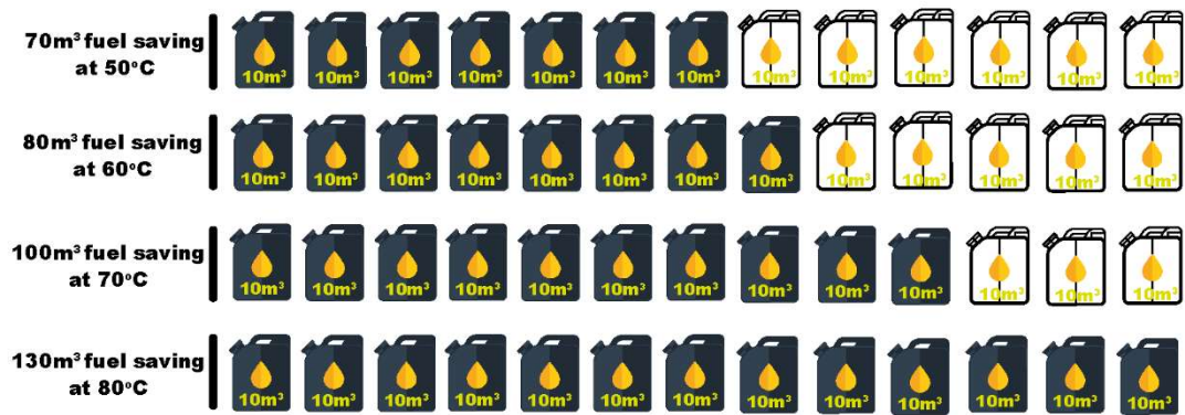
Figure 13 Annual fuel consumption savings with different PCM initial temperatures
