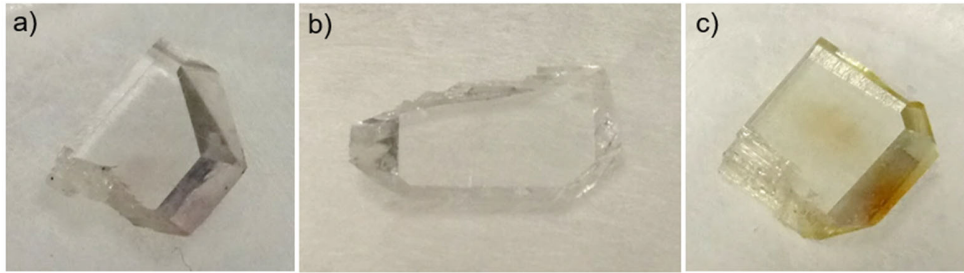
Fig. 5. a) Undoped KGdP, b) 1 at. % Ce:KGdP and c) 1 at. % Pr:KGdP single crystals just after continued X-ray irradiation.
