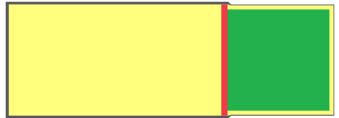
Fig. 1. Cross-section of the detector geometry used in the simulations. The modelled parts are: scintillation crystal (green), aluminium (grey), glass light guide (red) and air (yellow). (For interpretation of the references to color in this figure legend, the reader is referred to the web version of this article.)
