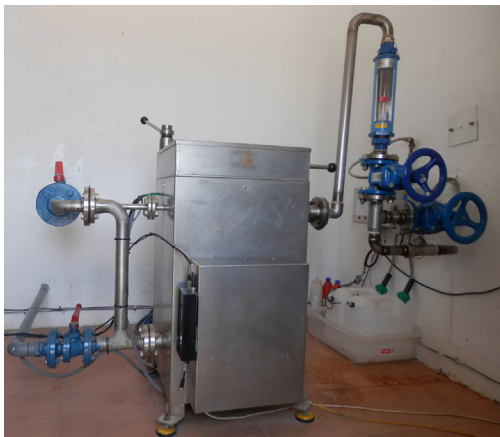
Fig. 1. Image (left) and scheme (right) of the water monitor. The Pb shielding is in the box represented by the dashed lines.
