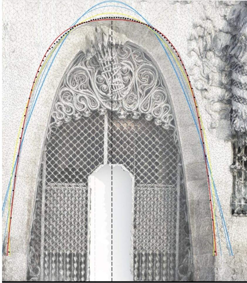
Fig. 6. Curve \gamma is shown in red over the study arch. Curve \delta is shown in yellow. The four remaining regression curves (parabola, hyperbola, catenary and hyperbolic cosine curve) are shown in blue.
