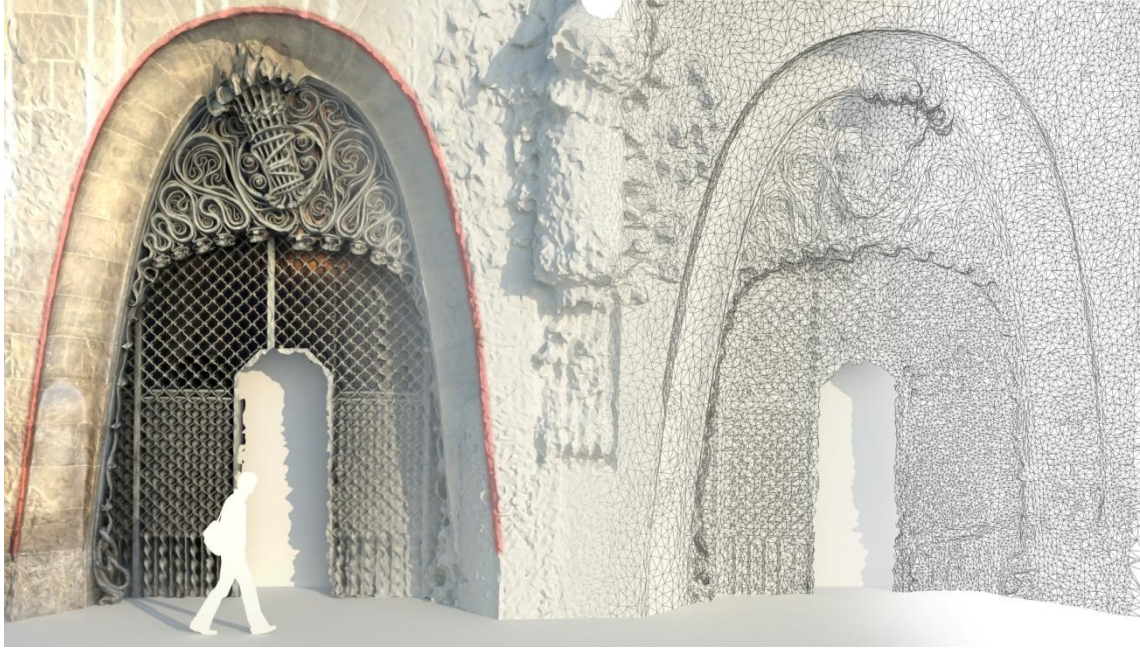
Fig. 3. Outline of the three-dimensional model of the study object created with PhotoScan software. The edge contour of the study arch is highlighted in red.
