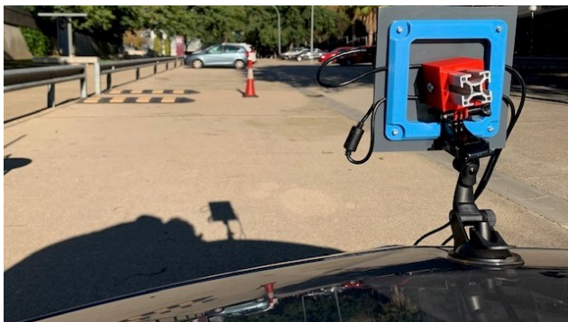
Fig. 19. Photography of scenario 3 with the rotating corner mounted on a safety cone near a guardrail and the radar mounted in a car.
