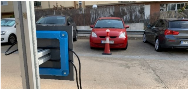
Fig. 16. Photography of scenario 2 with the rotating corner mounted on a safety cone in front of a car.
